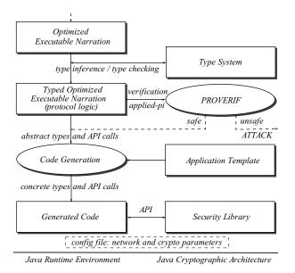
$\textbf{Figure 2.} \ \, \textbf{Compiler back-end (Type System, Code generator, Verification) and runtime support }$
