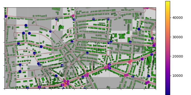
Fig. 4: Weighted placement. The covered area is smaller, but the samples per point are one order of magnitude higher.
