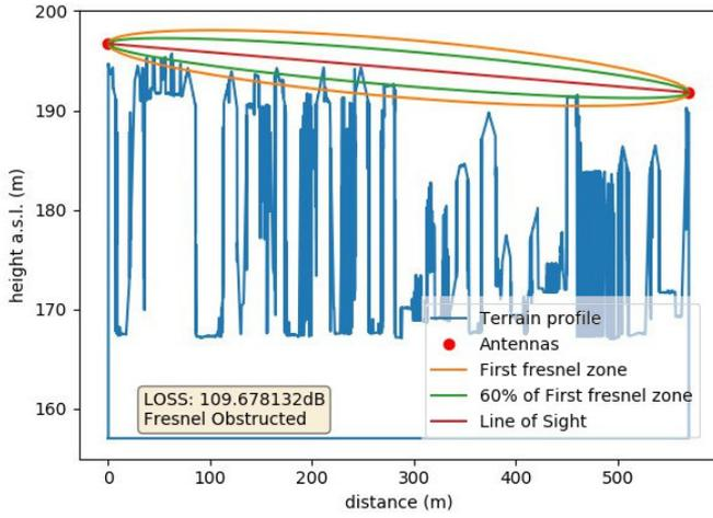
Fig. 1. Graphic representation of the elevation profile with LOS and Fresnel area.
